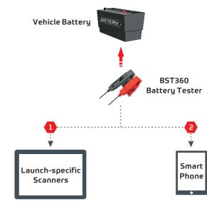
The scanner needs to be equipped with the BST360 module.
