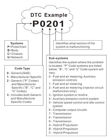
P0201 - Injector circuit malfunction, Cylinder 1
