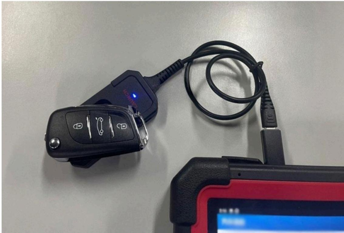
3. For car models without electronic keys, enter [Set type of wireless remote] to generate the corresponding key
