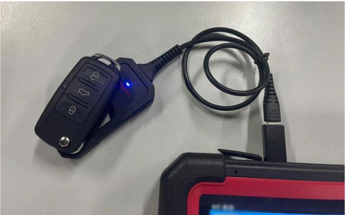
3. After the remote control is successfully generated, enter the [Set type of super chip] menu to generate the corresponding key chip.
